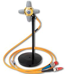
**Internal calibration data** The linearity adjustment data is by default stored inside the probe. In addition, the frequency response calibration data of the X-Y-Z axis can be stored as user correction data inside the probe. As a result there is no need to apply frequency dependent corrections for individual axis' in software anymore. This feature results in a high accuracy and ease-of-use.
