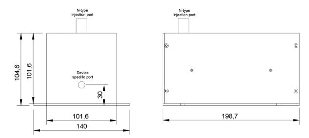
Each Radi Coupler® has a device specific connector for the EUT and AE-port. This connector is located at 30mm above the bottom plate of the CDN.
