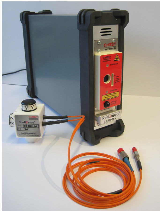
Figure 2: Beam shutter (red) on the RadiSupply® plug-in card (in the RadiCentre® system)
