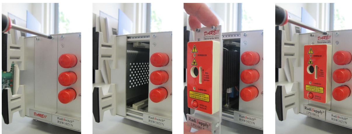
Figure 12: Example of a (RadiSupply® LPS1001A) plug-in card installation
