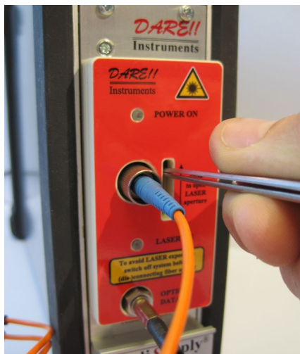
Figure 3: Opening the slide (left) and inserting the FC connector with the notch facing right (right)
