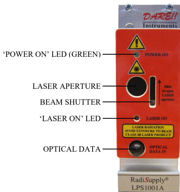
Figure 1: RadiSupply® plug-in card with beam shutter
