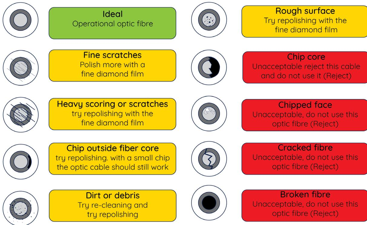
Reference figure for fibre maintenance
