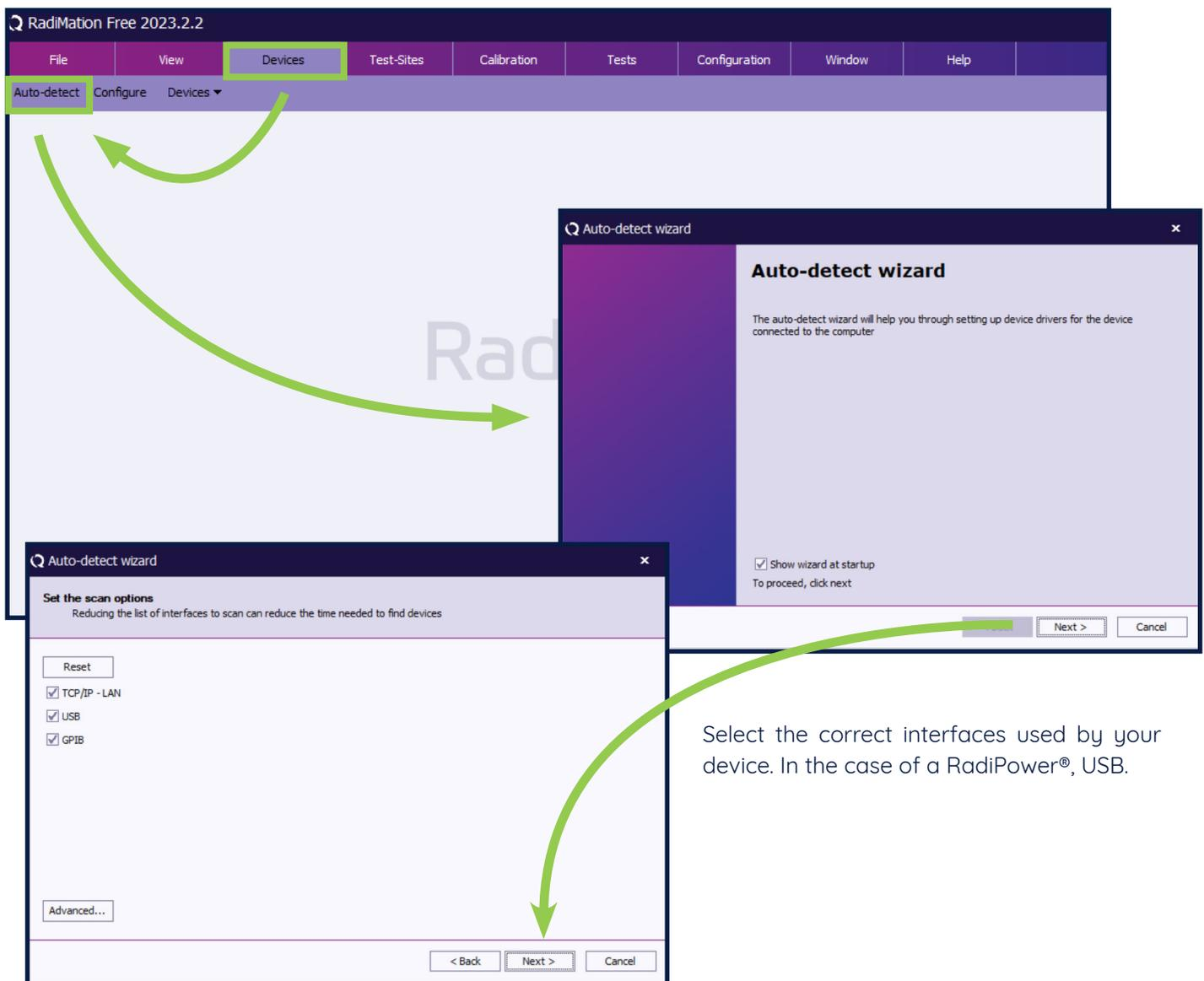
Select the correct interfaces used by your device. In the case of a RadiPower®, USB.
