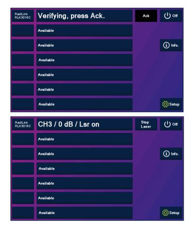
The RadiCentre will now prompt the message "verifying, press Ack." By pressing the ACK button whitin 2 seconds the RadiLink plugin card will beep and initialize the laser.
